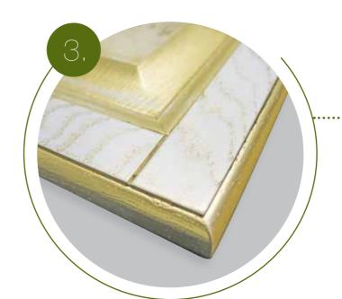
The patina is removed using a scotch-brite sponge, so it only remains in the wood grooves and pores.
