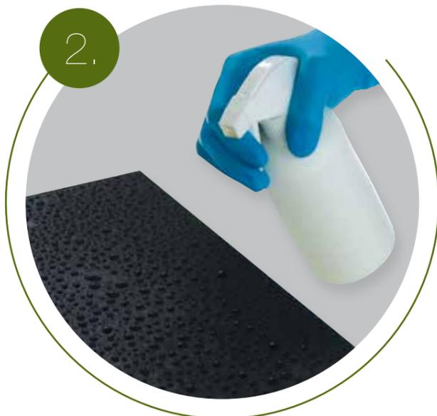
Do not sand the surface before spraying the drops. Using a spray bottle, apply the drops in the desired size and continue with shading.
