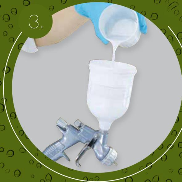
Use KOMBIHEL patina CROMÉ for shading or any other colour shade. Spray from one side only, so the drops are coloured on one side.
