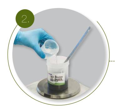
In step 2 the prepared paste mixture is dilluted in a prescribed ratio.
